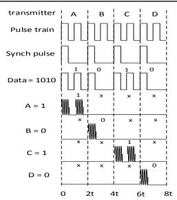
Figure 1: The Enhanced SPPM signal (Popoola *et. al.*, 2012)
